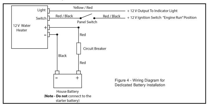
NOTE: For a dual battery system, Whale® recommends the use of a Battery Management System.
