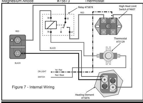
NOTE: Figure 7 depicts the internal wiring of this Water Heater. For advice on servicing any of the highlighted components please contact Whale® Support (Section 13) or a marine electrician.
